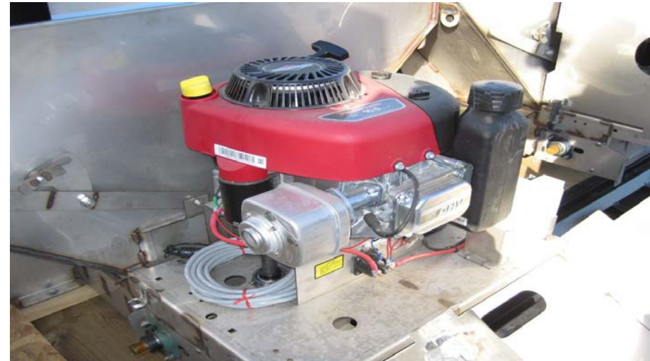
An average 10.5HP gasoline-powered salt spreader
